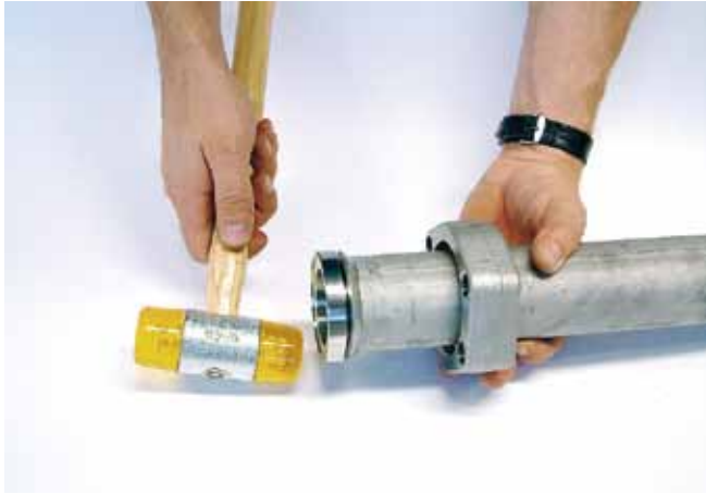
Fit the insert cone into the tube flare. If needed, tap gently with plastic or hide mallet.
