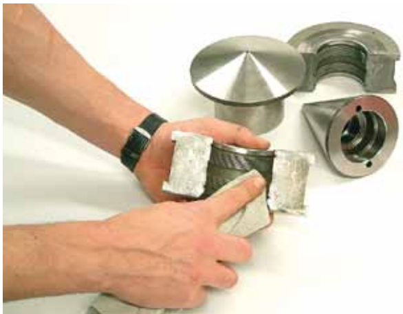
The flaring cone and dye is cleaned before beginning the flaring.
