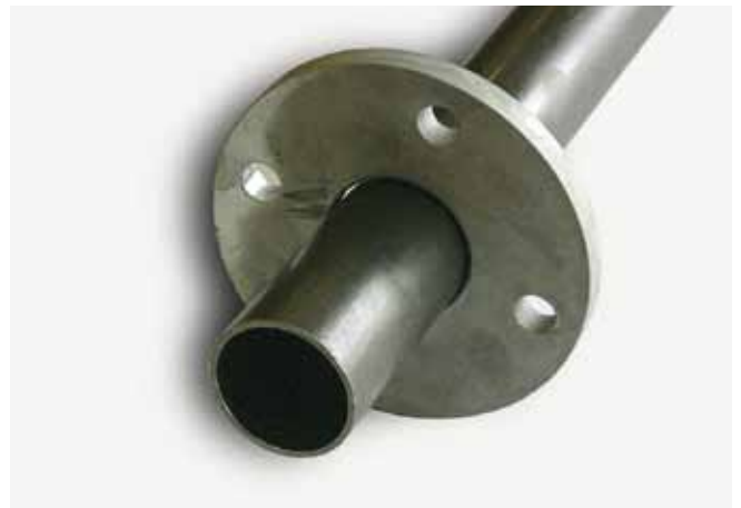
The flange is placed on the pipe end with chamfer facin outwards.
