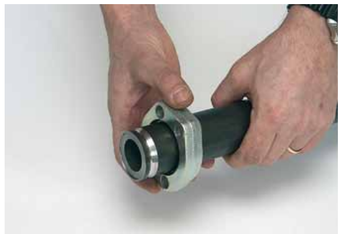
Install the flanges with the retain ring groove facing towards the end of the pipe. The original GS-flange has a GS-PIPING -text, marking of flange type and a charge number for traceability.
