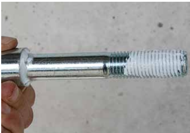
Lubricate bolt threads amply according to illustration. If tightened on bolt, lubricate bolt head compression face. If tightened on nut, lubricate nut on flange side.
