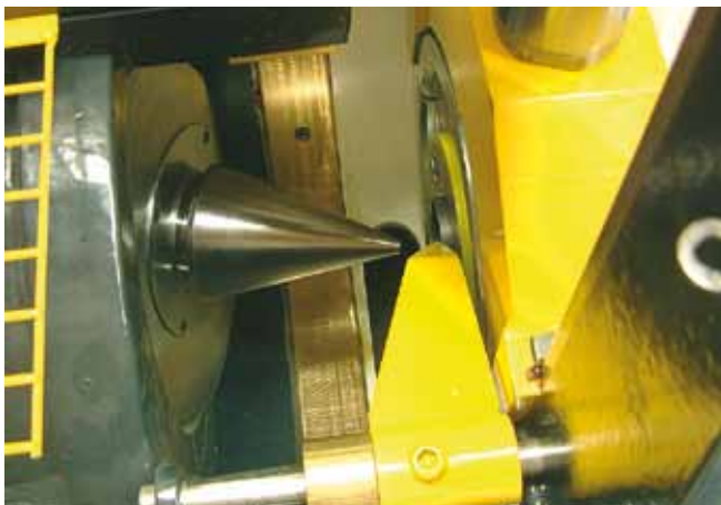
The pipe end is inserted into the dies with the correct flaring dimensions.
