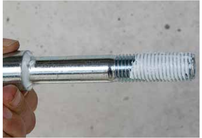
Lubricate bolt threads amply according to illustration. If tightened on bolt, lubricate bolt head compression face. If tightened on nut, lubricate nut on flange side.
